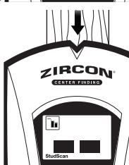
In cases of deeper studs (thicker walls), when the centre of the stud is located, only two bars will show on the Signal Strength Indicator and only the SpotLite® Pointer and middle segments of the Target Indication Bars will illuminate. If you still cannot locate a stud, try DeepScan® mode. Display will light green with the word "DeepScan" to indicate the mode.
