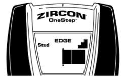
Continue sliding tool. When the centre of stud is located with three bars on the Signal Strength Indicator, the four Middle bars, centre indication, and SpotLite® Pointing System will all illuminate, and the buzzer will sound.
