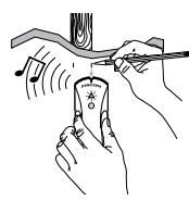
Continue scanning beyond the marked spot until the red EDGE light turns off. Slide unit in reverse direction to locate other edge of stud. Mark this second spot. The middle of the stud is centred between the two marks.
